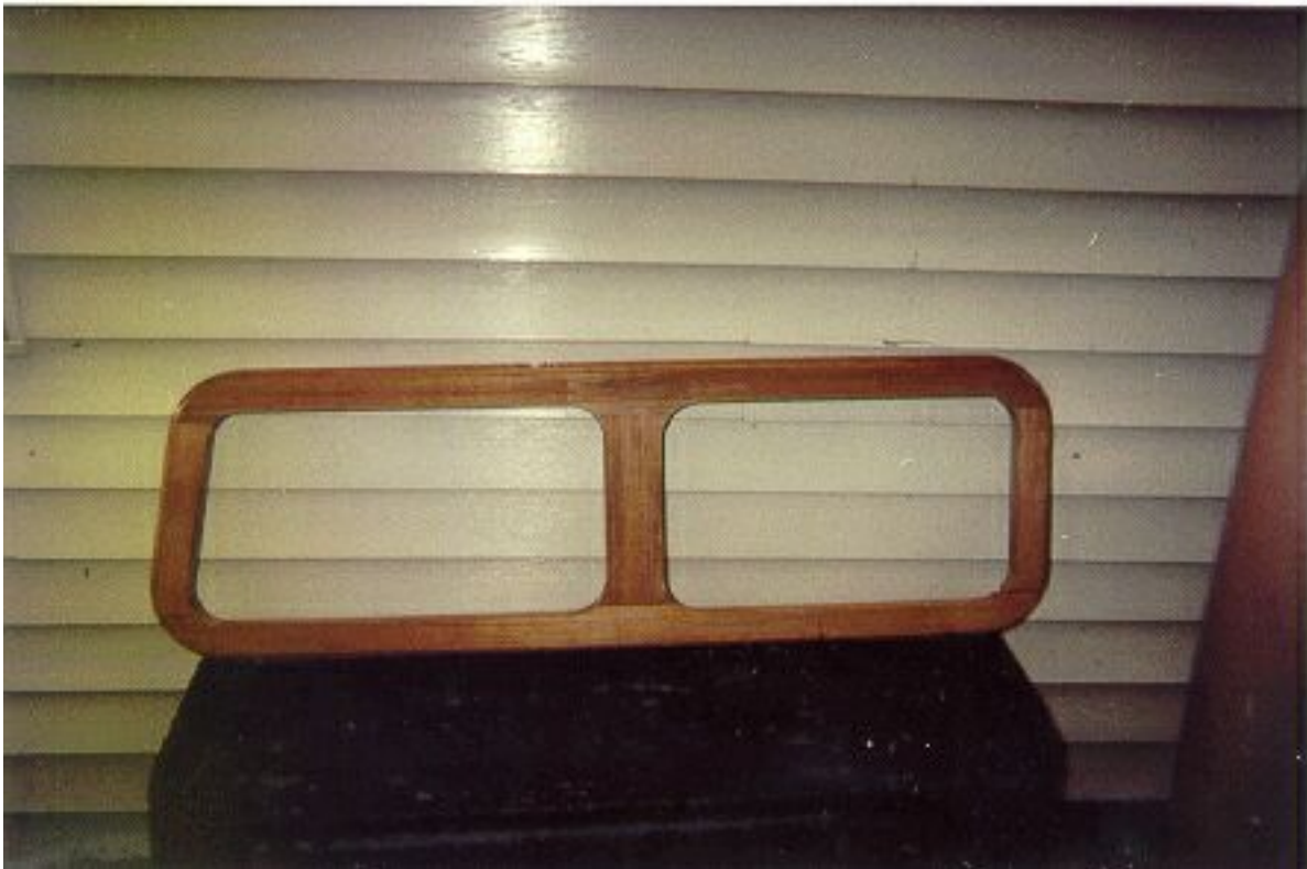
INSIDE VIEW OF FORWARD WINDOW FRAME
