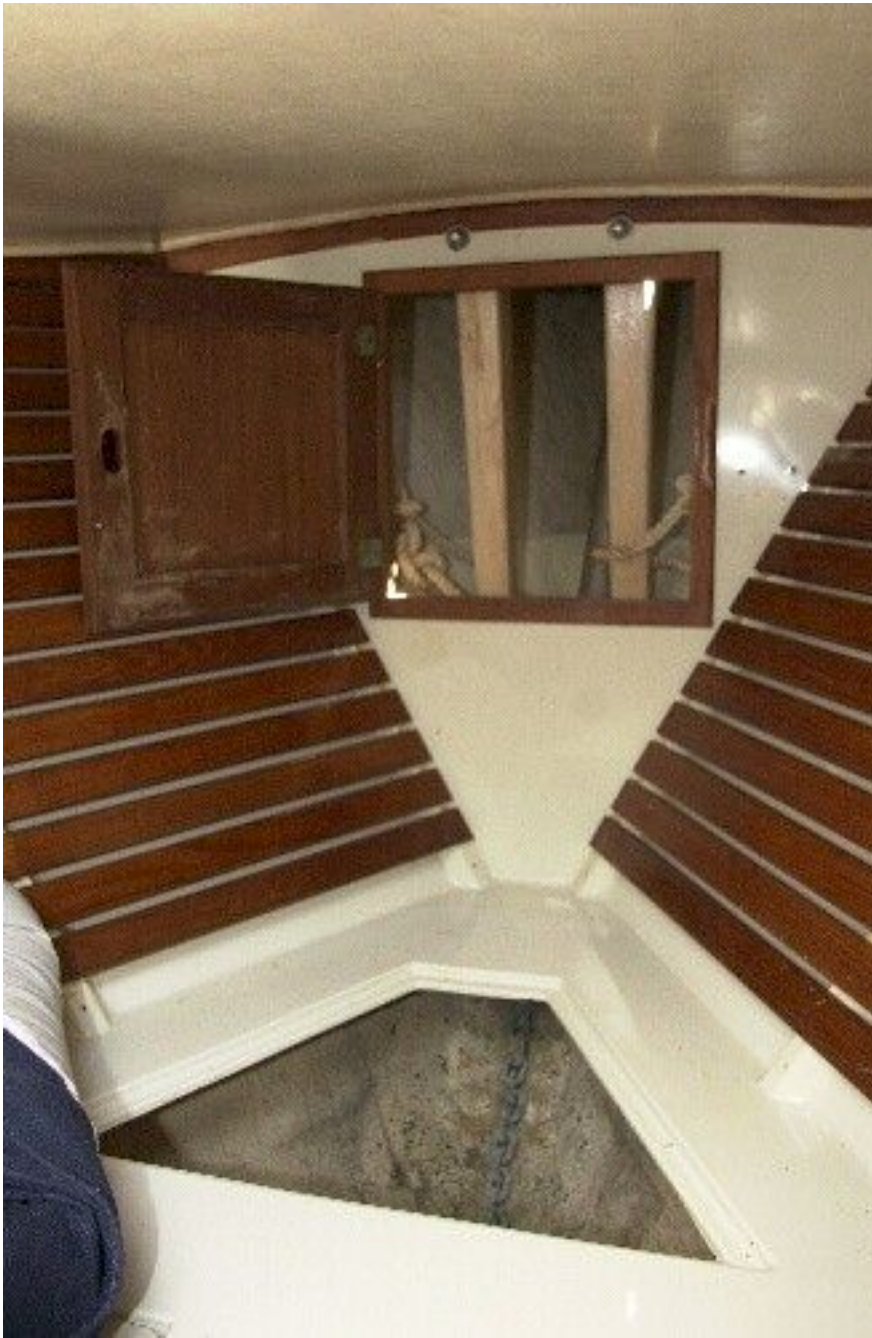
Close up of upper "rode" (i.e rope) locker with "naval" pipe to lower chain locker.
